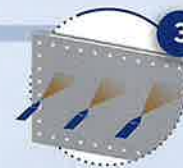
3 Shot blasting to SSPC SP-10/NACE2
